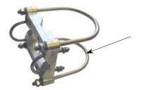
If the antenna boom is long enough, the clamp can be installed in a horizontal position and bigger pole diameter (such as 115 mm) can be afforded with U-bolts used as mark ④ on picture at left.
