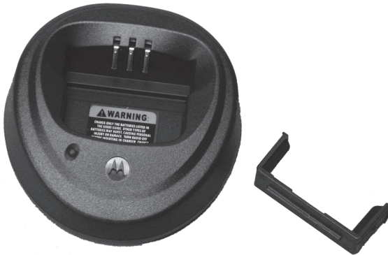
Figure 2 Battery Locating Rail removed
